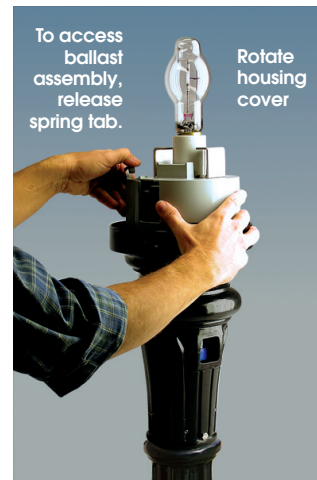
LUMINAIRE BASE WITH BALLAST HOUSING AND SOCKET
