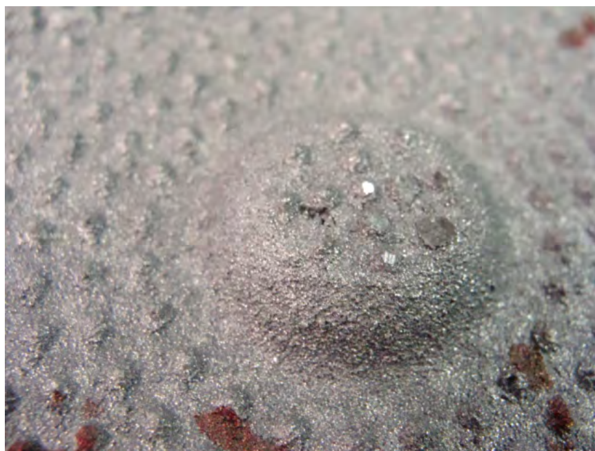
Photo No. 4 – Typical Damage to the Dome After 27 J Impact at Ambient Temperature
