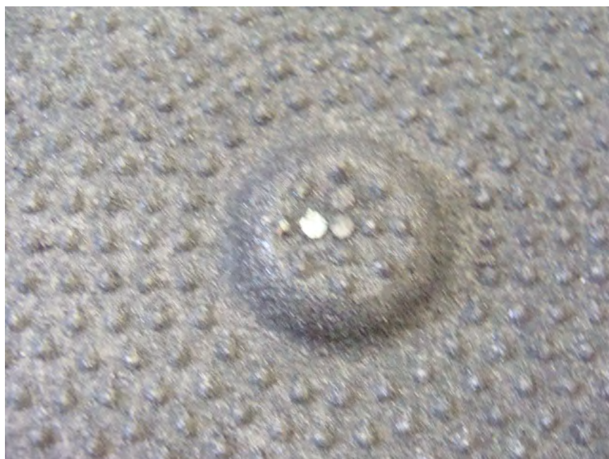
Photo No. 6 - Typical Damage to the Dome After 27 J Impact at -4° C Temperature
