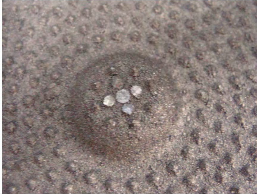
Photo No. 7 - Typical Damage to the Dome After 54 J Impact at -4° C Temperature
