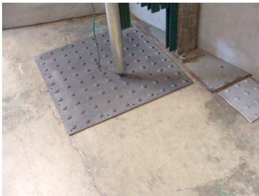
Photo No. 3 – Positioning of the Panel for the Impact
