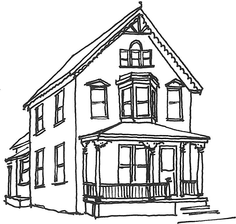
The character of the simple residence has been altered by the addition of inappropriate ornamentation
